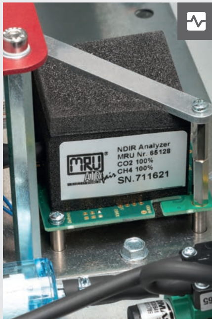
NDIR-bench for \text{CH}_4/\text{CO}_2 analysis, for biogas and landfill gas measurements
